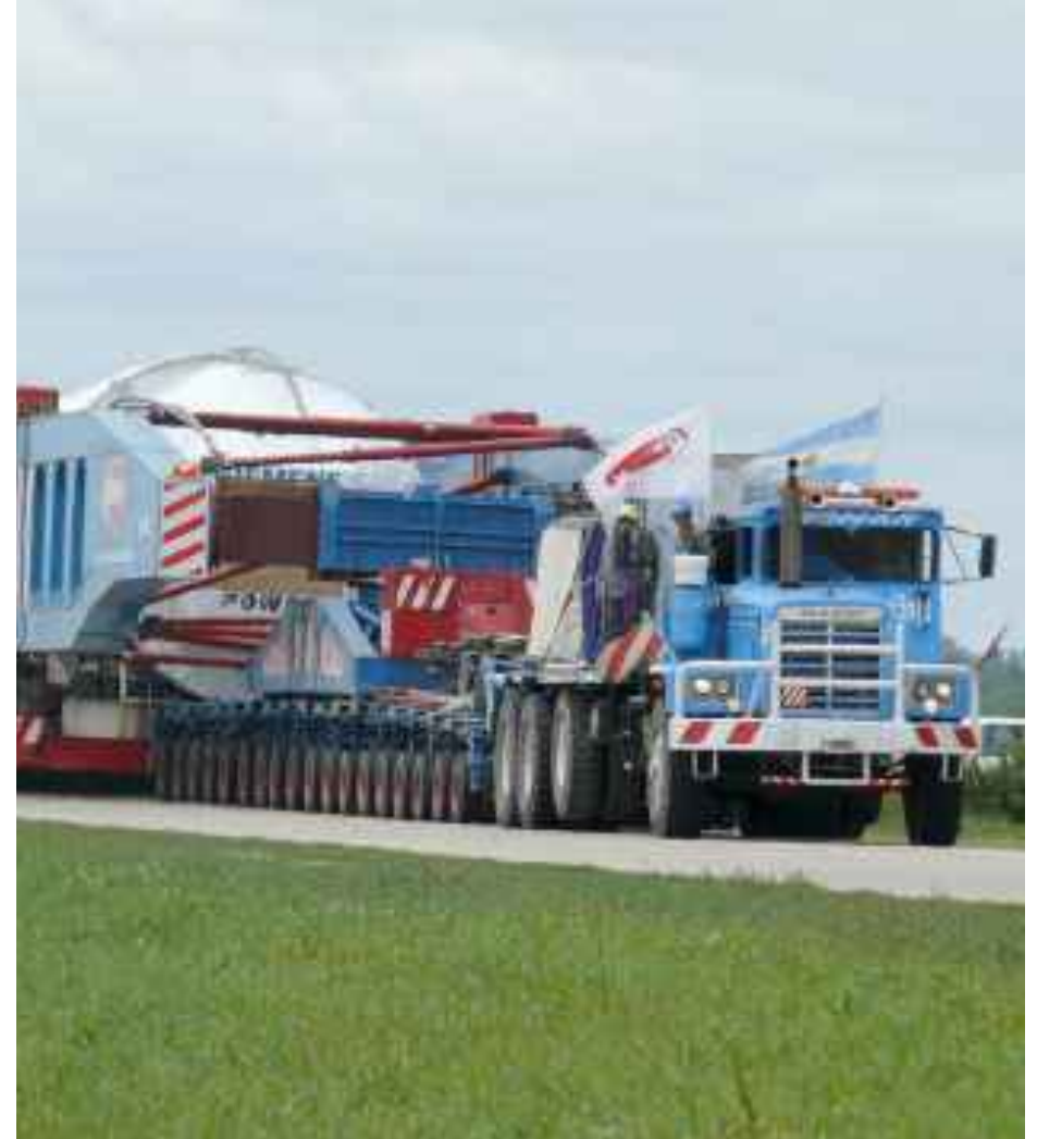
TRANSPORTATION OF A 318 TONS SIEMENS TURBINE FROM ZARATE TO A POWER PLANT IN SAN MARTIN TIMBUES, SANTA FE
